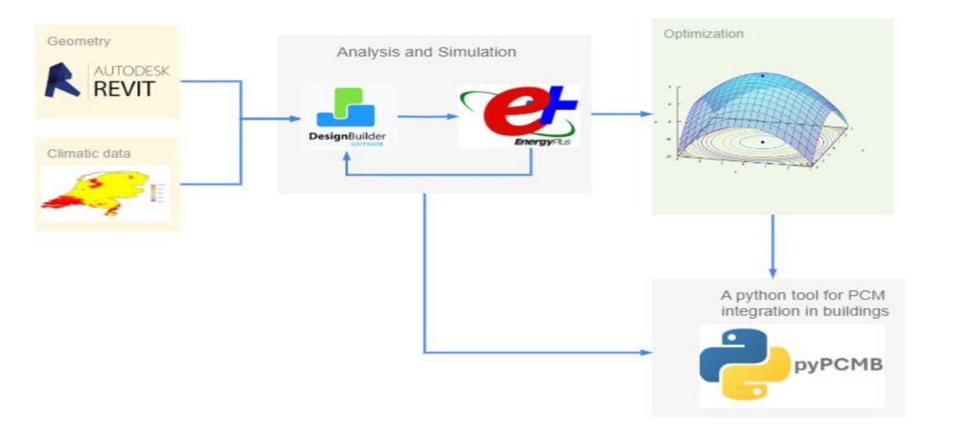
Autodesk Revit was used to design a typical Dutch terrace building, with parameters from [1]. EnergyPlus weather data for Amsterdam, Netherlands, informed our simulations. We explored eight scenarios: six with PCM integrated into walls, and two with air and XPS insulation. EnergyPlus simulations offer robust modeling of phase change materials (PCMs) in building components. Validated by [2], EnergyPlus employs a conduction finite difference algorithm, allowing users to
