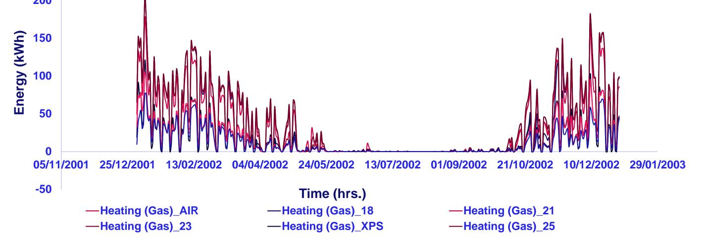
The heating load graph highlights the superior performance of the XPS-insulated wall in reducing heat loss. This aligns with expectations, as winter ambient temperatures typically don't reach PCM melting points, minimizing phase changes. Numeric values denote PCM phase change temperatures.
